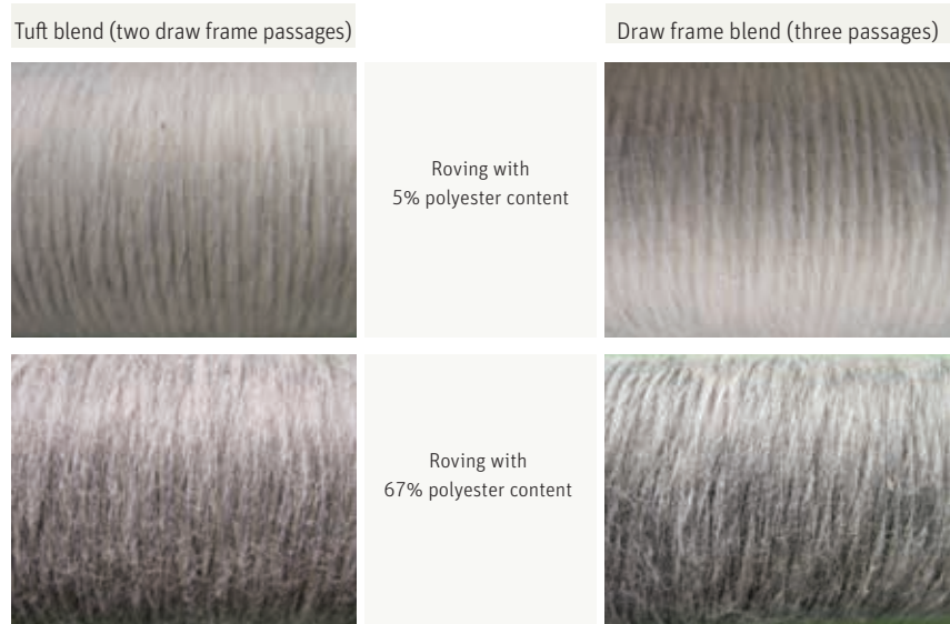
Fig. 24: Comparison of the homogeneity of tuft versus draw frame blend with an additional draw frame passage
