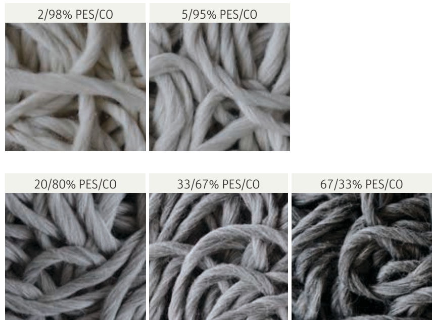
Fig. 18: Homogeneity of the tuft blend after the roving frame
