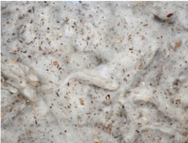
Fig. 5: When spinning waste or material with high short-fiber content the direct rotor spinning process is the optimal solution.
