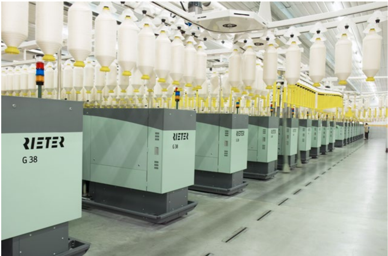
Fig. 11: The ring spinning machine G 38 uses minimal energy thanks to double-sided suction and energy-efficient components.
