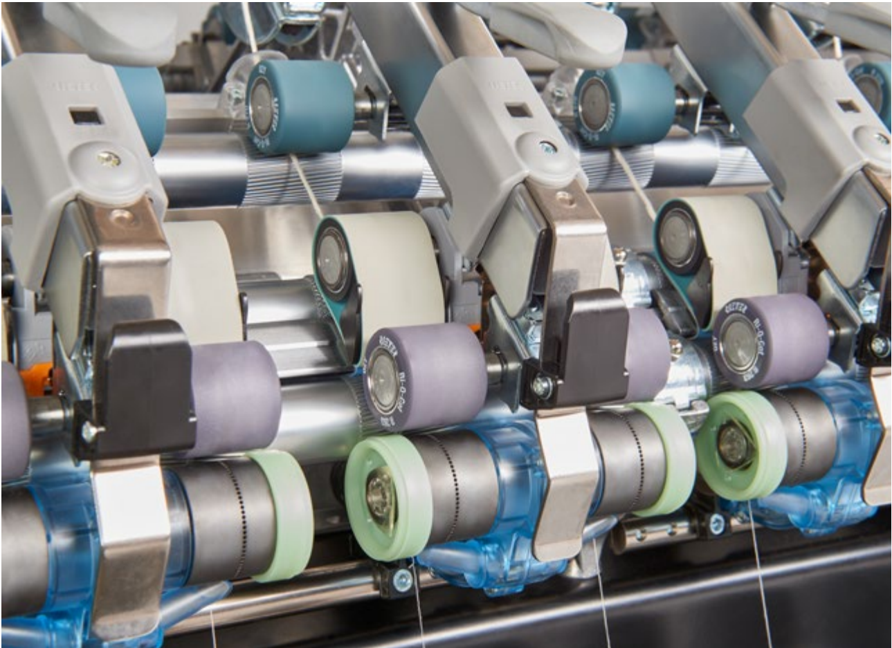
Fig. 15: Efficient use of resources by upgrading an existing ring spinning machine with COMPACTdrum.
