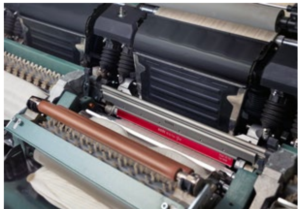
Fig. 6: The comb E 90 secures gentle and controlled fiber treatment what results in best raw material utilization.
