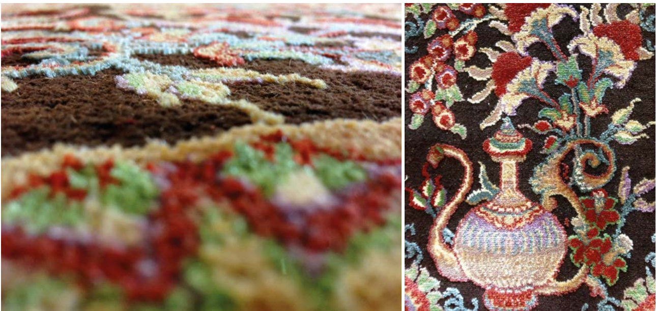
Fig. 5 and 6: Carpets with 3D effect with high-shrinkage pile used for the dark background and low-shrinkage pile used for the flourish design
