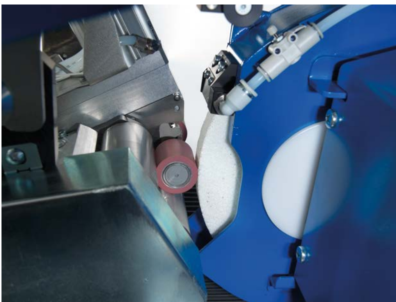
Fig. 1: Grinding position of a top roller with a diameter of 30 mm
