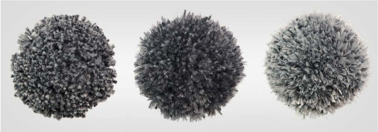
Fig. 7: Various shrinkage level combinations and their different appearance within the pile
