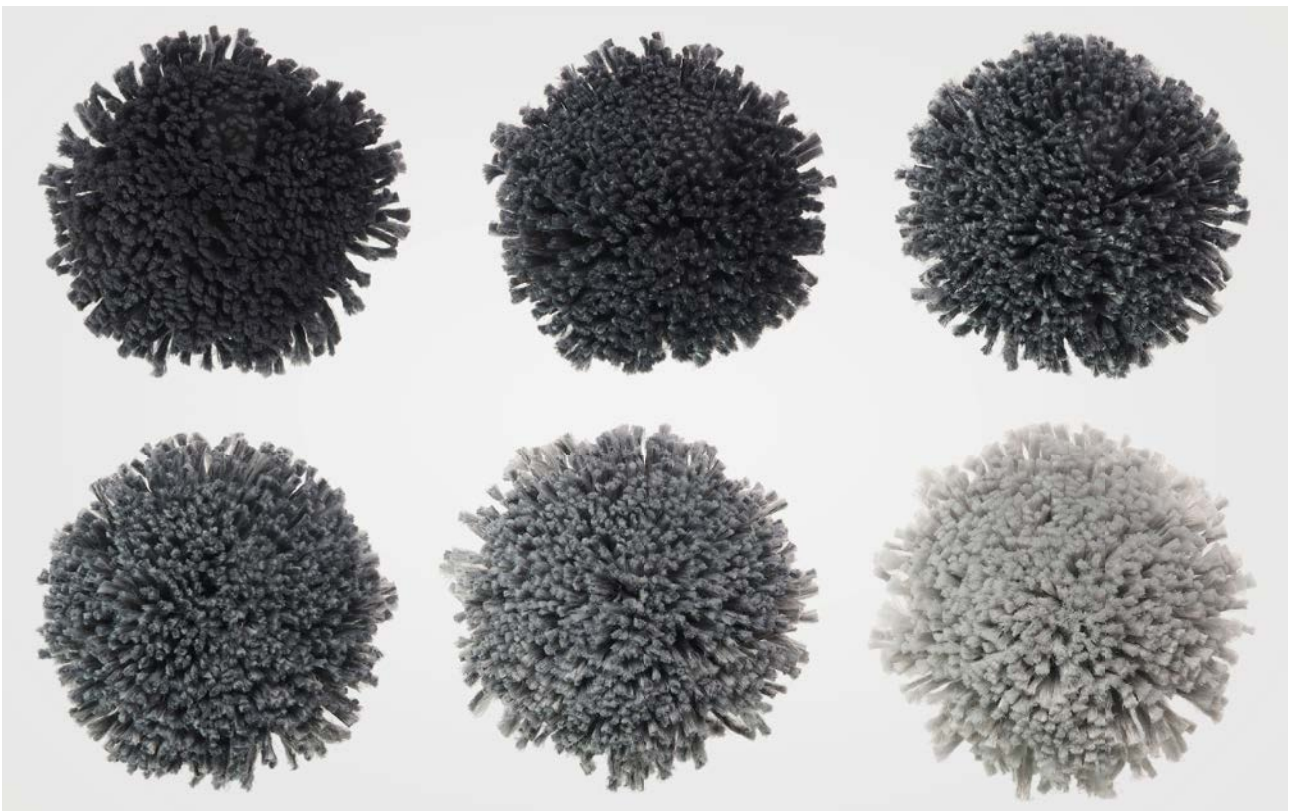
Fig. 3: Color flexibility of pile with only two supply colors
