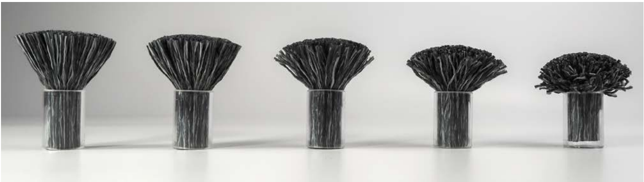
Fig. 4: Different shrinkage levels ranging from a minimum of 4% to a maximum of 65%.
