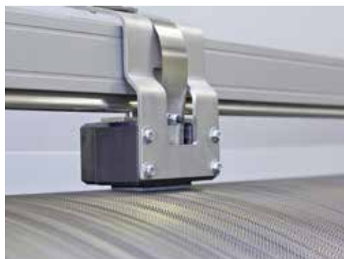
Fig. 4: ASG – Doffer resharpener device
