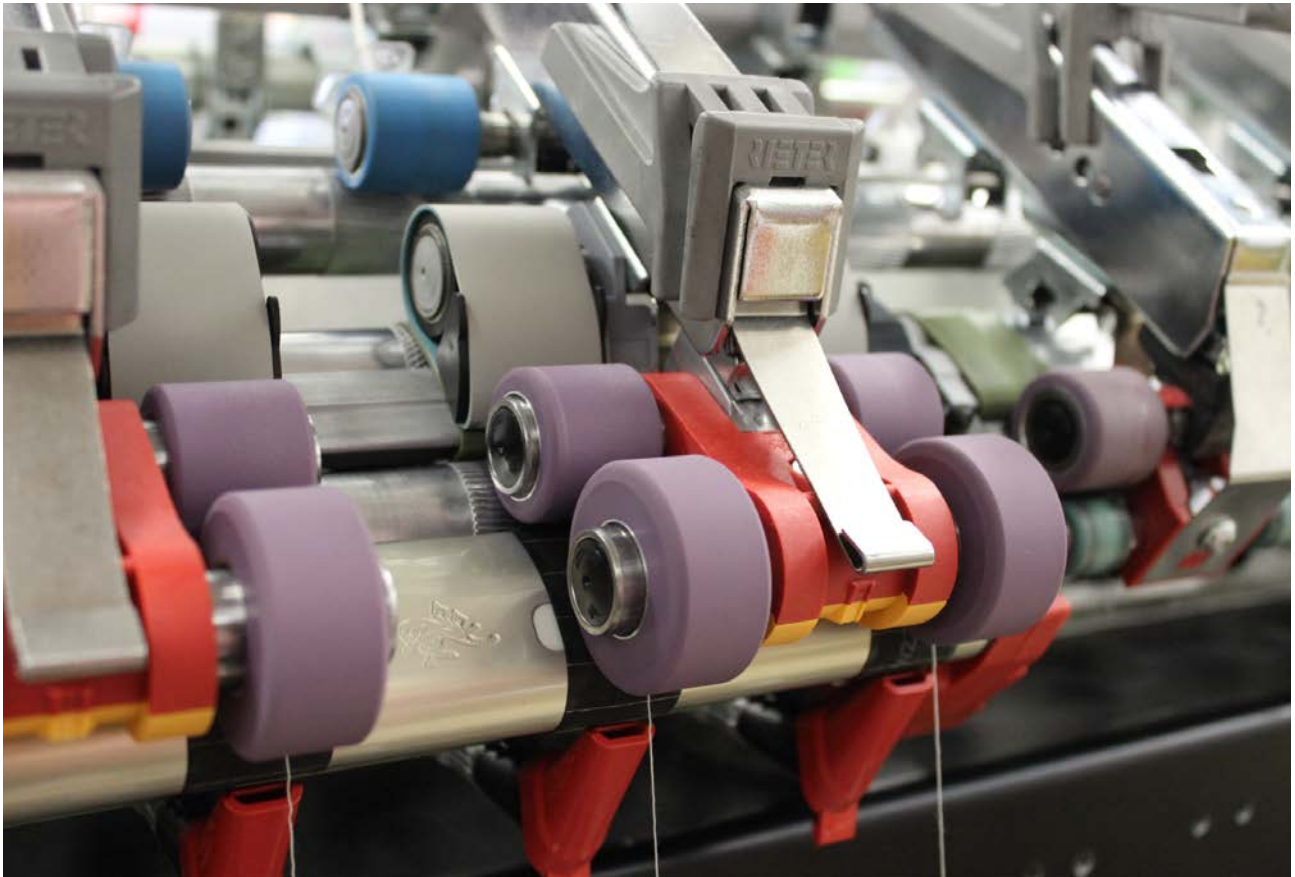
Fig. 1: COMPACTeas spinning system
