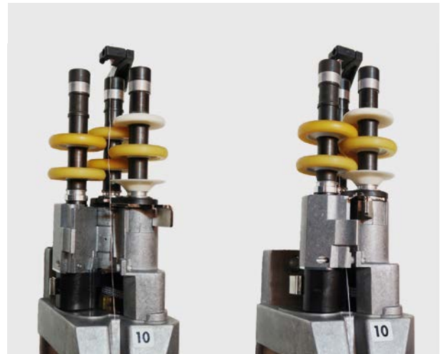
Fig. 6: SSM spindle GS50, open-close view
