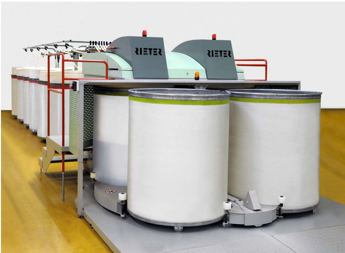
Fig. 7 Blends of cotton with man-made fibres are increasing. The SB-D 22 draw frame is ideally suitable for mixing the fibres.
